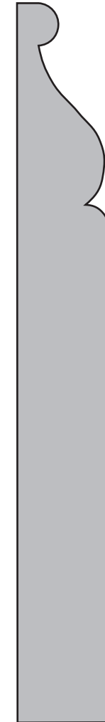
BCB500 5/8 X 5 1/4 in. Also Available: BCB300 5/8 X 3 1/4 in. BCB400 5/8 X 4 1/4 in. BCB700 5/8 X 7 1/4 in. BCB925 3/4 X 9 1/4 in.
